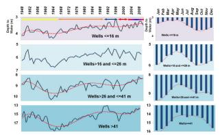
Figure 6. Mean annual depth to static water level variations for various well depths from 1948 to 2010 and the corresponding mean monthly variations
