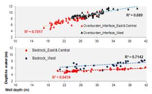
Figure 5. Relation between mean yearly well depth and depth to static water level, a) overburden (glacial sediment) and interface wells; b) bedrock wells
