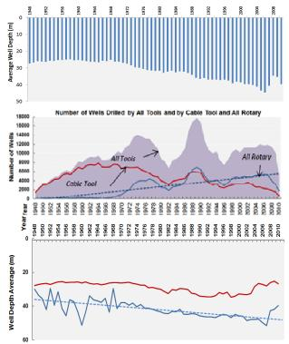
Figure 4. a) Average annual well depth variations for Southern Ontario 1948 to 2010 (upper figure); b) Number of wells drilled and drill method of all Ontario (middle figure); and c) Comparison of well depth over time for cable tool and rotary drilled wells of all Ontario (lower figure)
