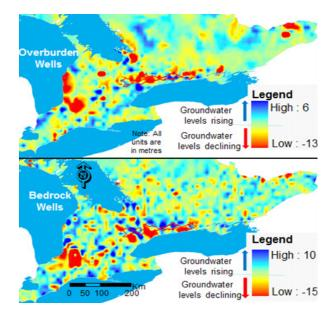
Figure 2. The integrated (average) measured depth to water levels from 1948 to 2010
