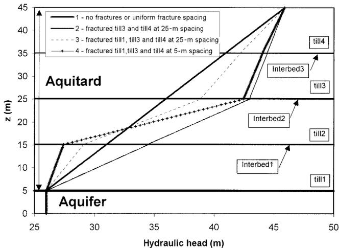
**Fig. 9** General aquitard/aquifer system showing relation between FRACTRAN calculated hydraulic head and depth at  $x=500$  m
