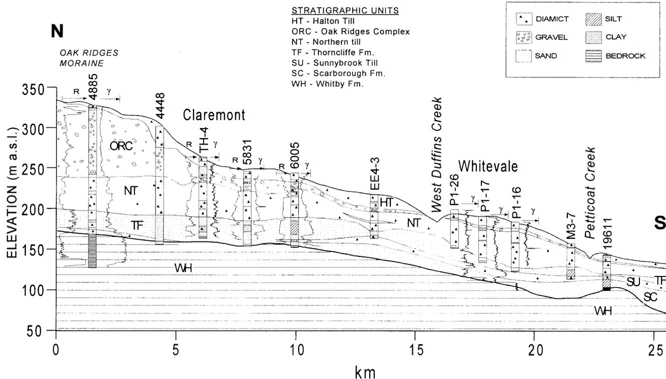
**Fig. 2** North-south cross section showing subsurface geology and hydrostratigraphy of the south slope of the Oak Ridges Moraine and study area. Borehole geophysical resistivity ( $R$ ) and gamma ( $\gamma$ ) logs are shown where available. See Fig. 1 for cross-section location. (After Boyce 1997)
